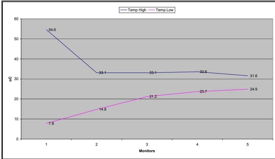
Table 56: Temperature Highs and Lows, KV 9, Sept. 12, 2004-Nov. 27, 2004
